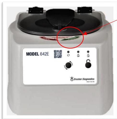
Peel back the right side of the label located at the latch. Reveal the opening underneath the label, insert a pen and pull the mechanism towards the front of the centrifuge.
